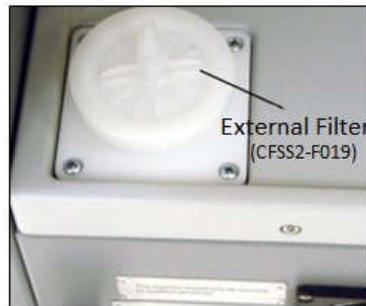
Figure 9.1: External Filter Installed
