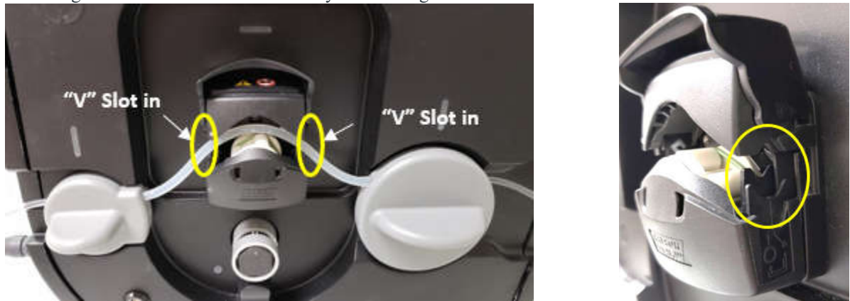
Figure 7.4.2.1.1 Irrigation Tubing Installation
