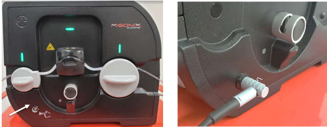
Figure 7.13.4 Wired Footswitch Connection to Console
