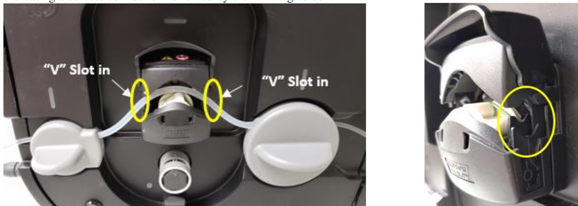
Figure 7.4.2.1.1 Irrigation Tubing Installation
