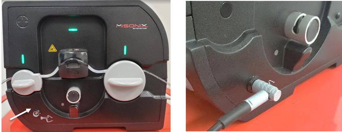
Figure 7.14.3 Wired Footswitch Connection to Console
