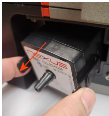
Figure 11.2.2: Pull out filter
