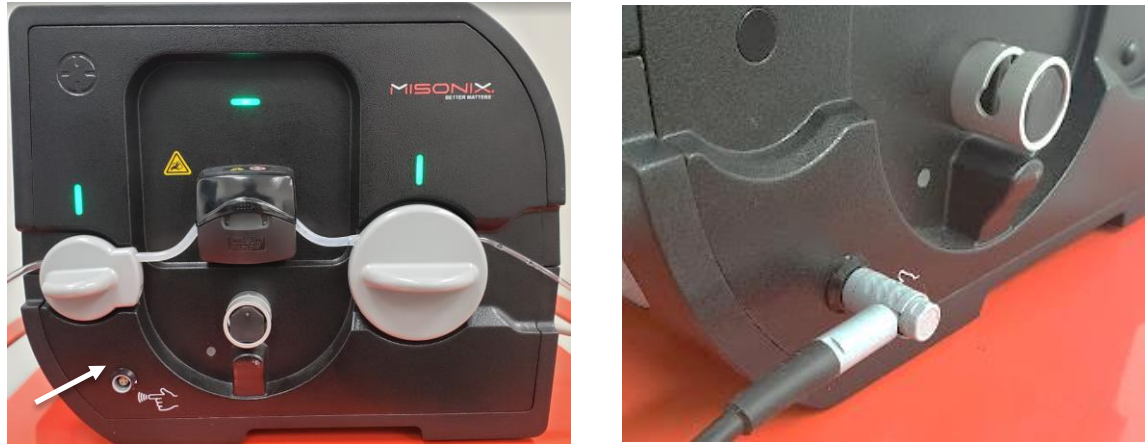
Figure 7.14.3 Wired Footswitch Connection to Console
