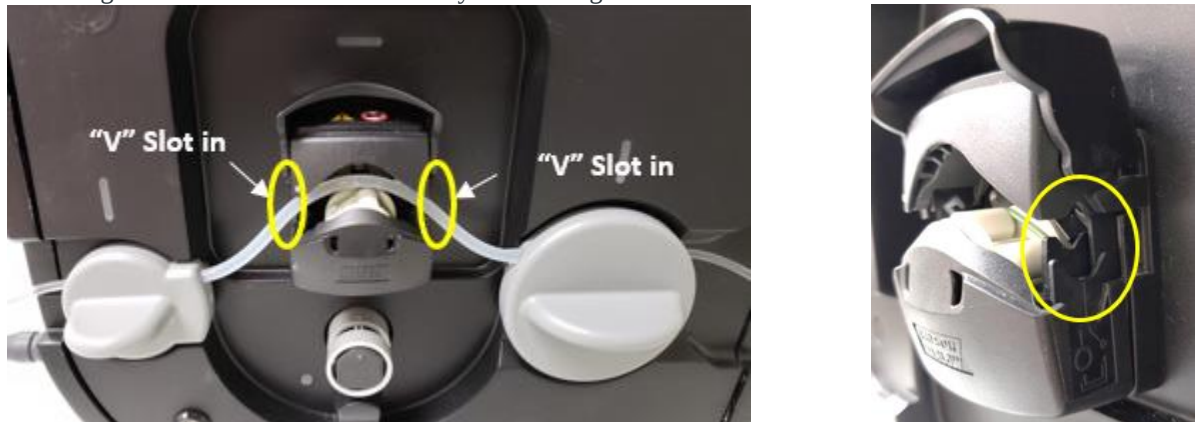
Figure 7.4.2.1.1 Irrigation Tubing Installation
