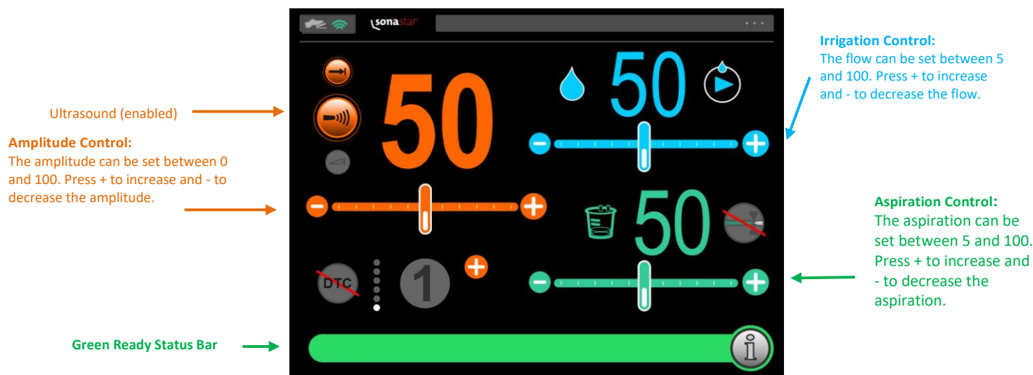
Figure 7.8.2 Default Main Screen (SonaStar Handpieces) with Ultrasound Enabled
